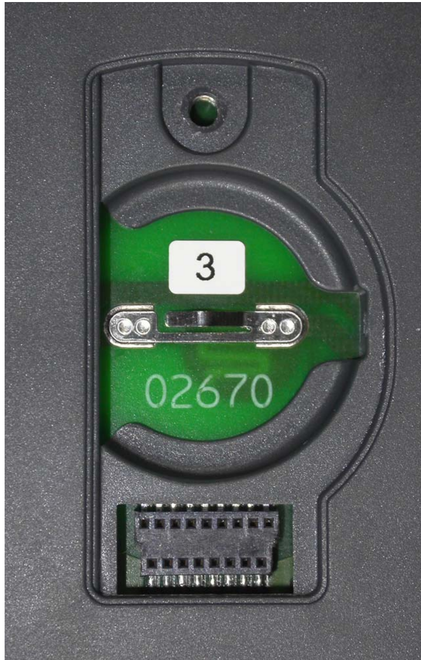
Internal photo Battery case
