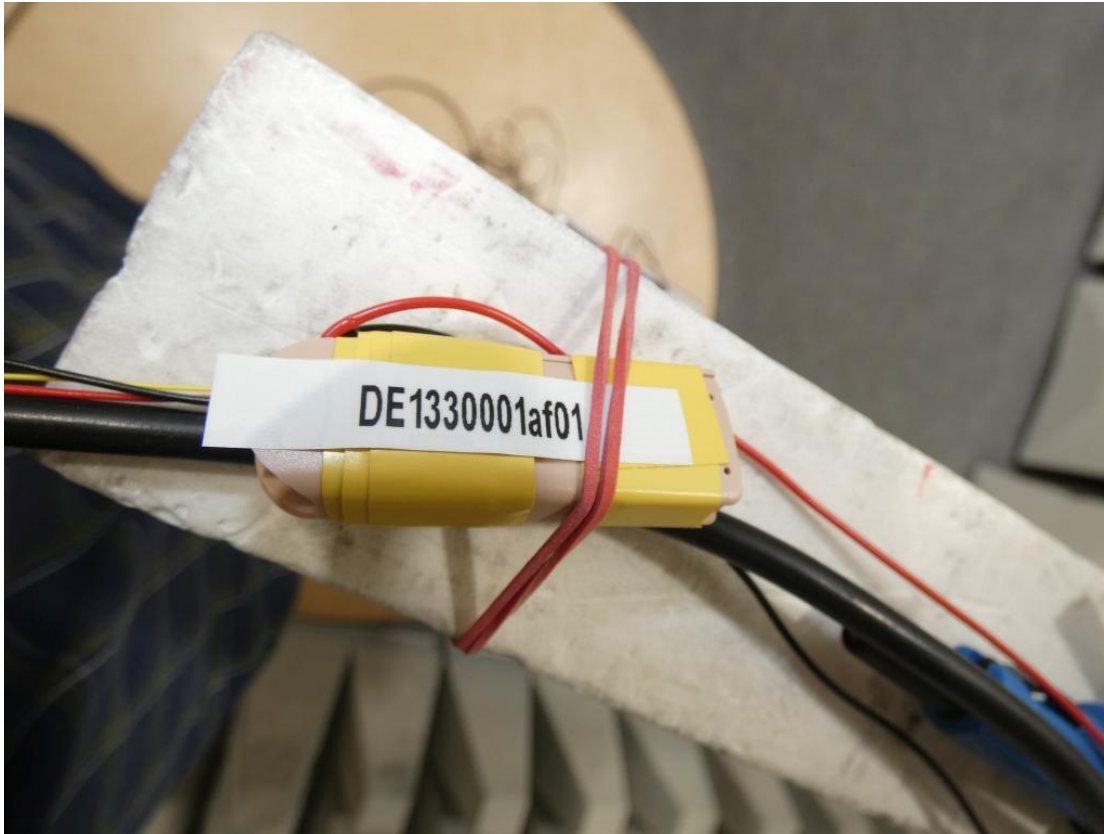
Photo 5: Test setup for radiated measurements, detailed view (stand alone setup, 1 GHz – 24 GHz; FCC 15c247)
