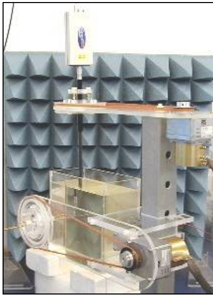
Figure 1. Spherical isotropy jig showing probe, dipole and box filled with simulated brain liquid(see Ref [2], Section A.5.2.1)
