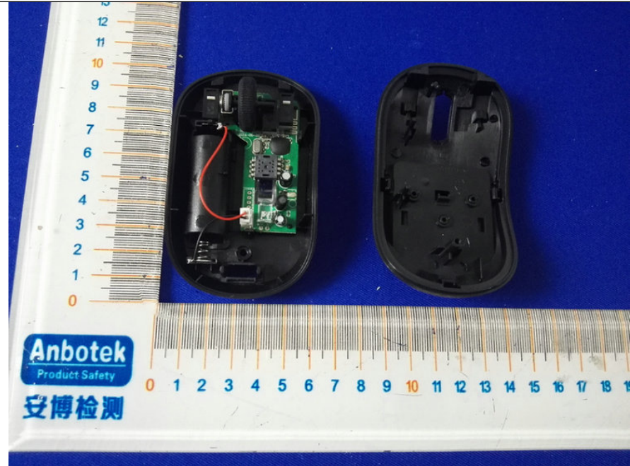
1. Figure The EUT-Inside View
