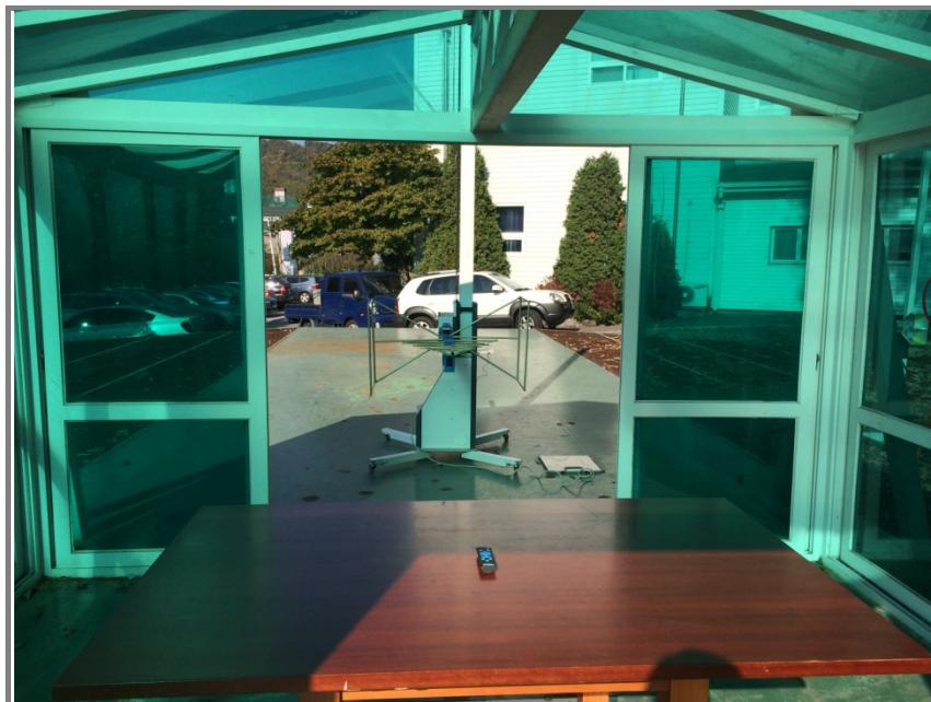
**Photo of radiated spurious emission at above 1 000 MHz**
