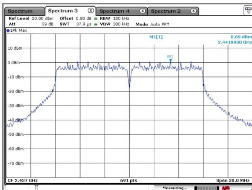
**Emission level measurement 1**
