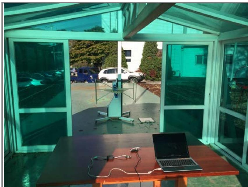
**Photo of radiated spurious emission at above 1 000 MHz**
