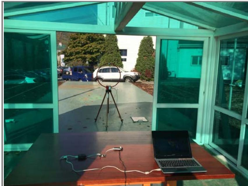
**Photo of radiated spurious emission at 30 MHz ~ 1 000 MHz**
