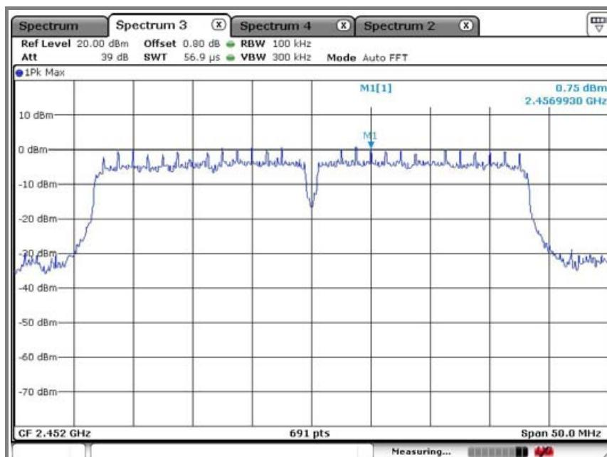
**Emission level measurement 1**
