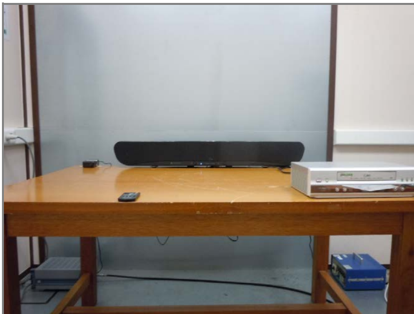
Photo of Conducted emission at below 30 MHz
