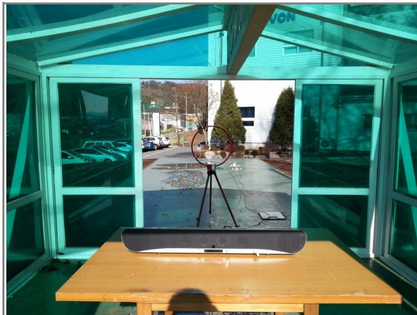
**Photo of radiated spurious emission at 30 MHz ~ 1 000 MHz**
