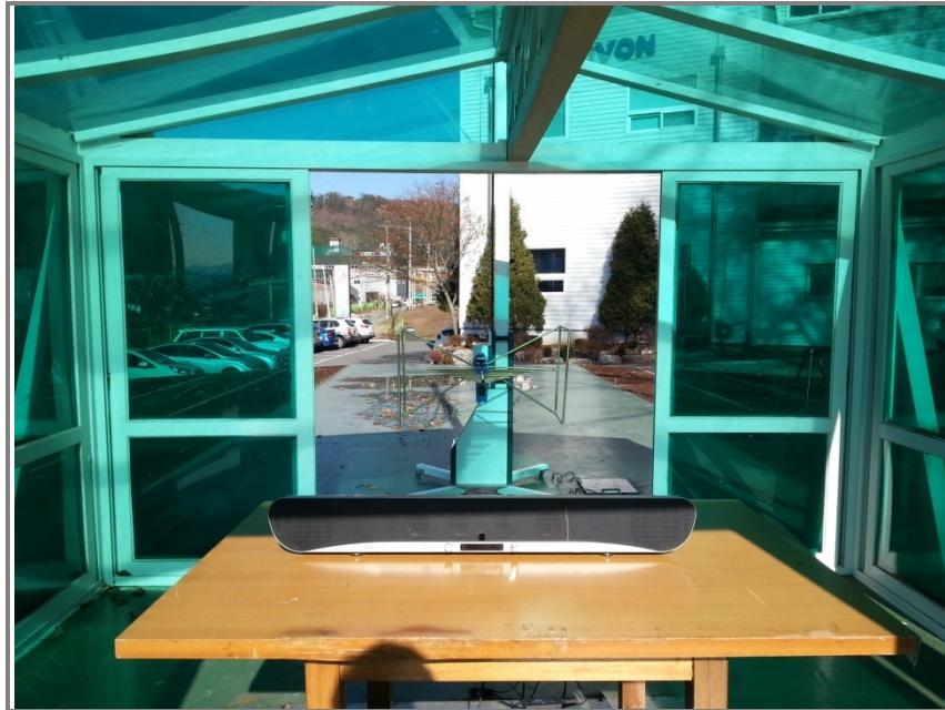
**Photo of radiated spurious emission at above 1 000 MHz**
