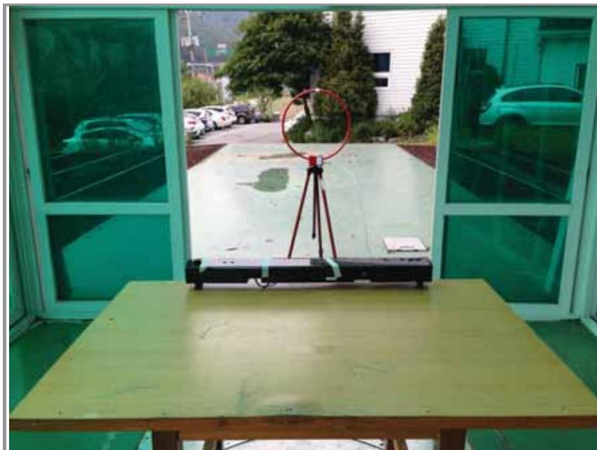
**Photo of radiated spurious emission at 30 MHz ~ 1 000 MHz**
