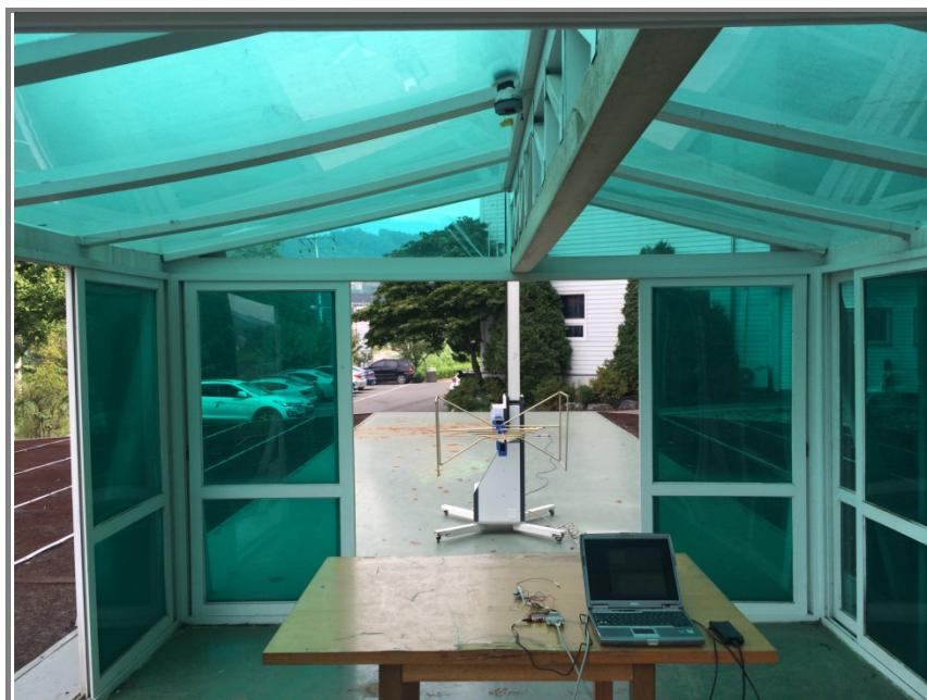
**Photo of radiated spurious emission at above 1 000 MHz**
