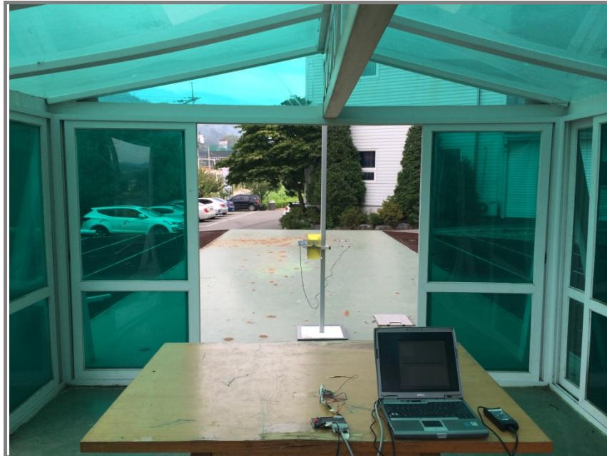
**Photo of Conducted emission at below 30 MHz**
