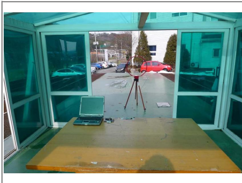
**Photo of radiated spurious emission at 30 MHz ~ 1 000 MHz**
