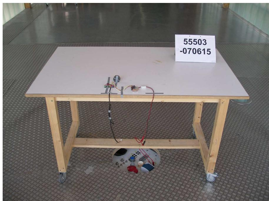
**Test setup for radiated emission measurement
