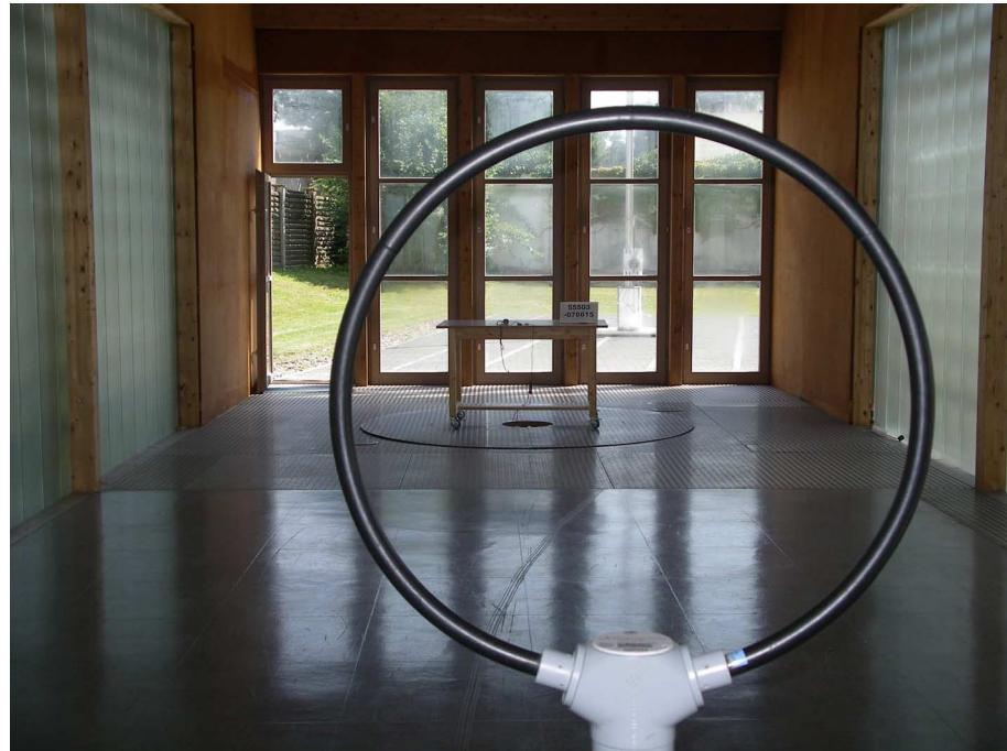
Note: Same test setup used as for radiated emission measurement 30 MHz - 1GHz
