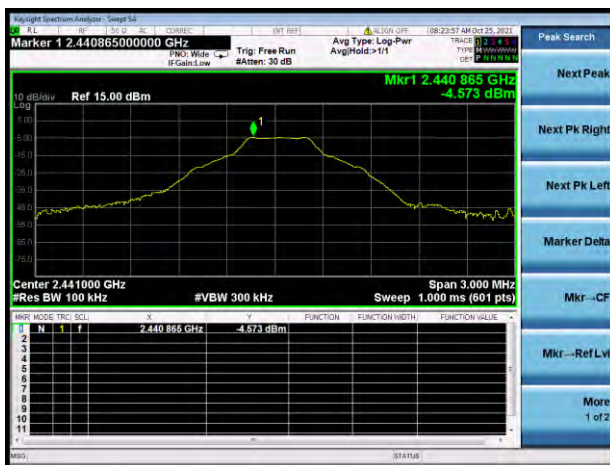
GFSK MIDDLE CHANNEL, CARRIER LEVEL
