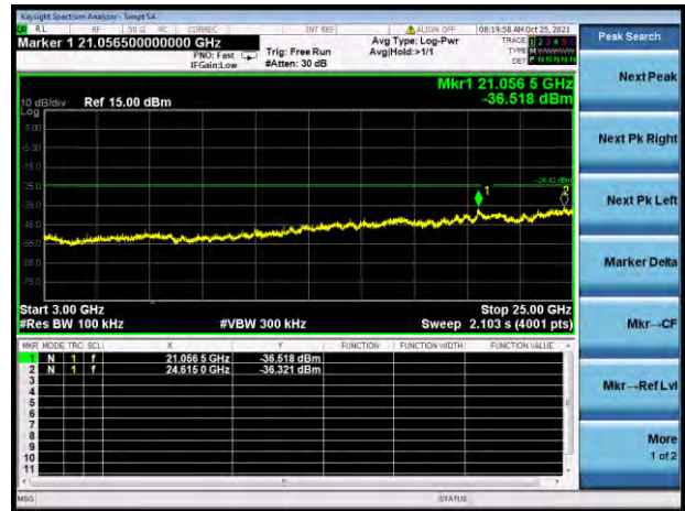
GFSK LOW CHANNEL, SPURIOUS 3 GHz ~ 25 GHz
