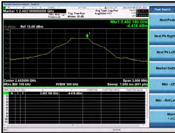
GFSK LOW CHANNEL, CARRIER LEVEL
