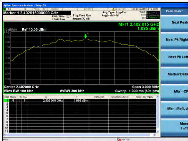
GFSK (BLE 2Mbps) LOW CHANNEL, CARRIER LEVEL
