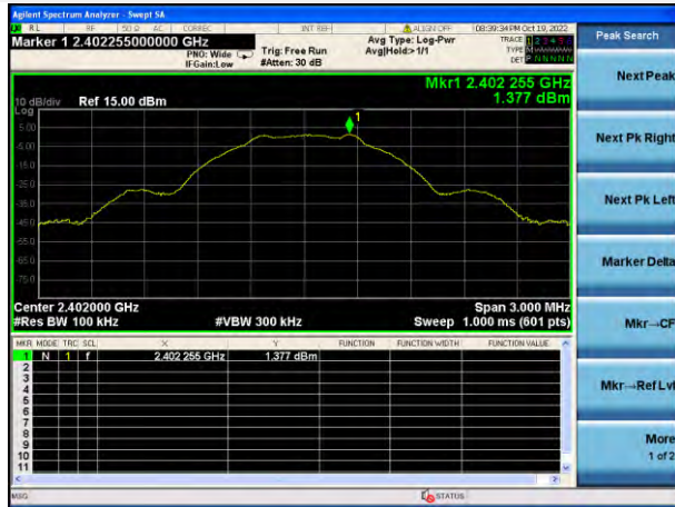
GFSK (BLE 1Mbps) LOW CHANNEL, CARRIER LEVEL
