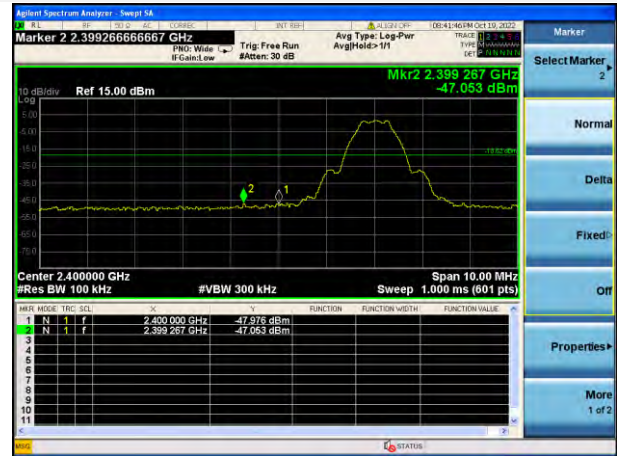
GFSK (BLE 1Mbps) HIGH CHANNEL, BAND EDGE
