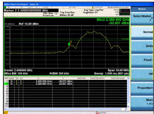
GFSK (BLE 2Mbps) LOW CHANNEL, BAND EDGE
