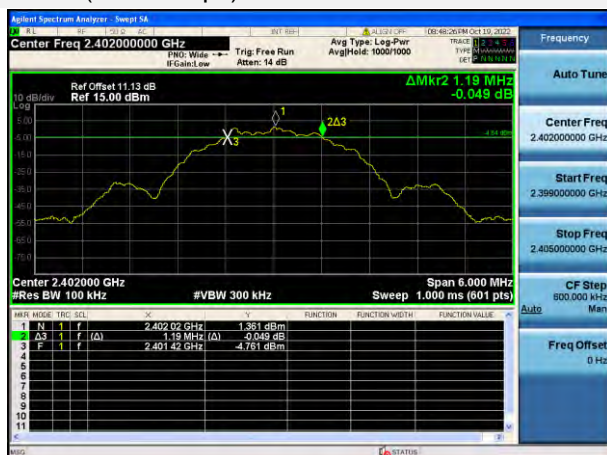
GFSK (BLE 2Mbps) LOW CHANNEL
