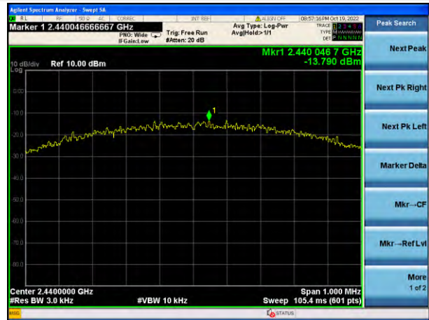
GFSK (BLE 1Mbps) MIDDLE CHANNEL
