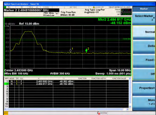
GFSK (BLE 1Mbps) HIGH CHANNEL, BAND EDGE
