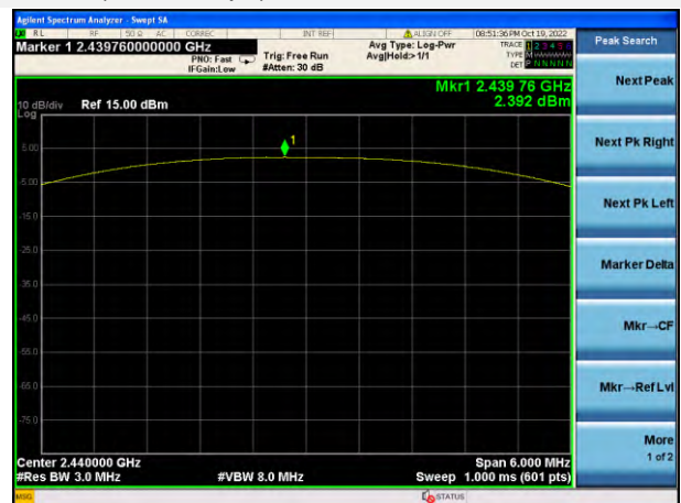
GFSK (BLE 2Mbps) MIDDLE CHANNEL
