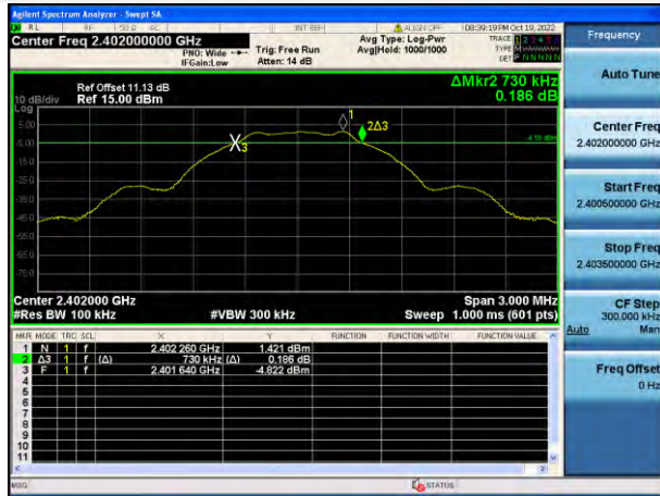
GFSK (BLE 1Mbps) LOW CHANNEL
