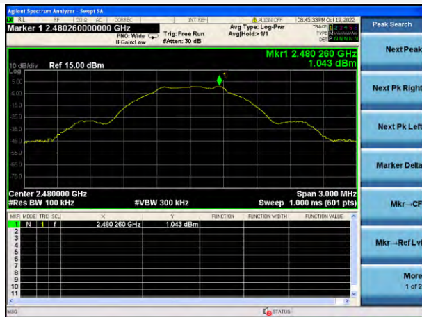
GFSK (BLE 1Mbps) HIGH CHANNEL, CARRIER LEVEL
