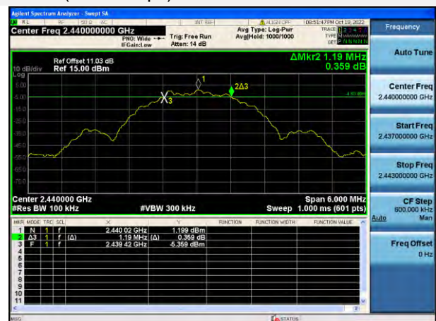
GFSK (BLE 2Mbps) MIDDLE CHANNEL
