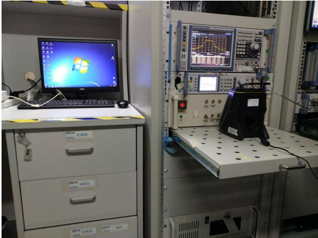
Conducted Test- 2.4G ISM Band( GFSK modulation)
