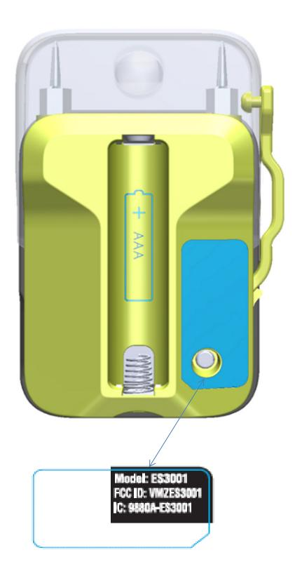
Label to be placed on back of device next to battery compartment.
