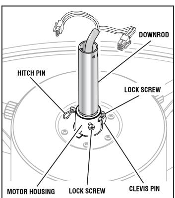
■ Carefully feed the fan's electrical wiring through the motor housing cap, then install the cap as shown.
