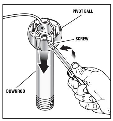
■ Remove the retainer pin from the downrod.
