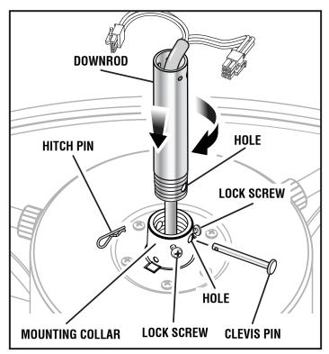
■ Thread the downrod into the motor housing until it bottoms out, then back it out until the hole in the downrod aligns with the hole in the motor housing. Be careful not to twist the electrical wiring when tightening.
