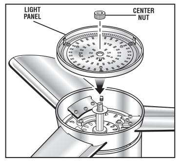
Insert the LED power lead into the socket on the light panel. Make sure the connection is securely seated, then flip the entire fan assembly right-side up to complete the rest of the assembly process.
