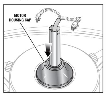
■ Carefully feed the fan's electrical wiring through the canopy screw cover ring and canopy, then install the cover ring and canopy on the downrod as shown.
