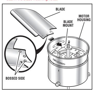
Install the lock washers and blade screws and tighten to secure the blade in place.
