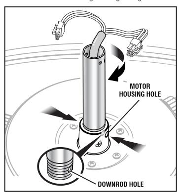
■ Install the clevis pin through the holes in the motor housing and the downrod, then reinsert hitch pin. Retighten the lock screws to secure.
