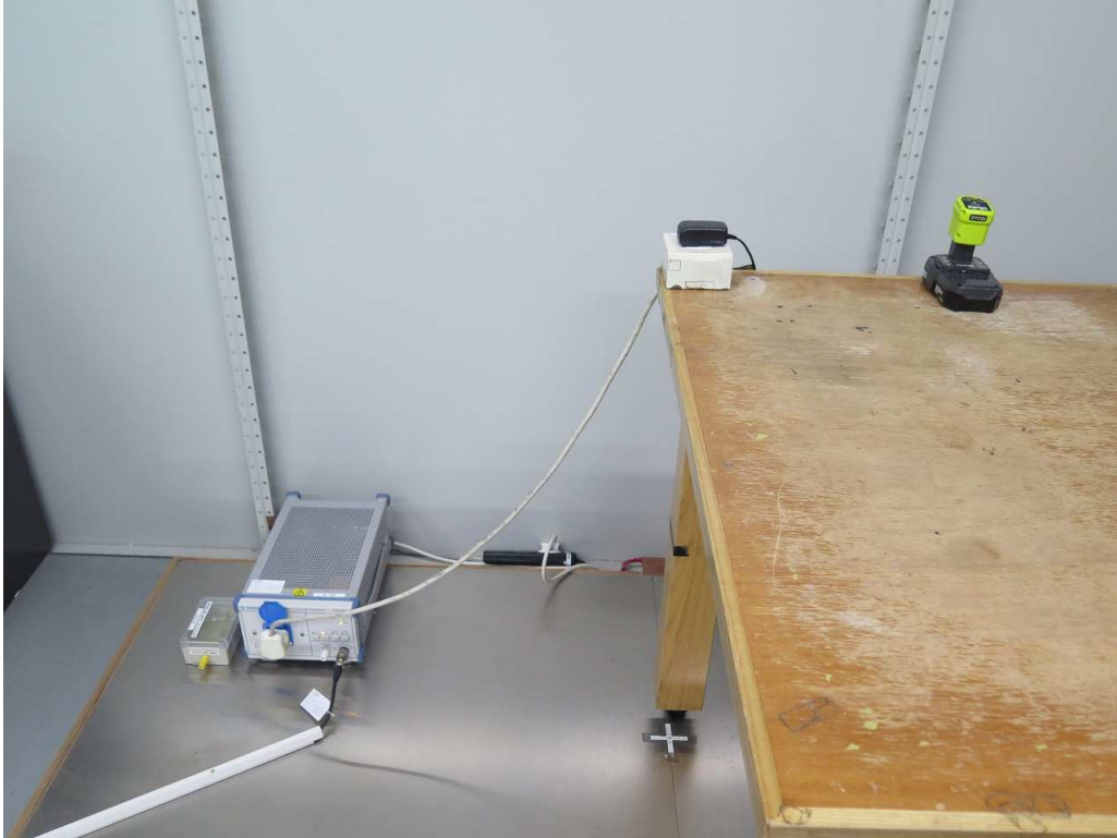
Line-conducted emission (front view, charging)
