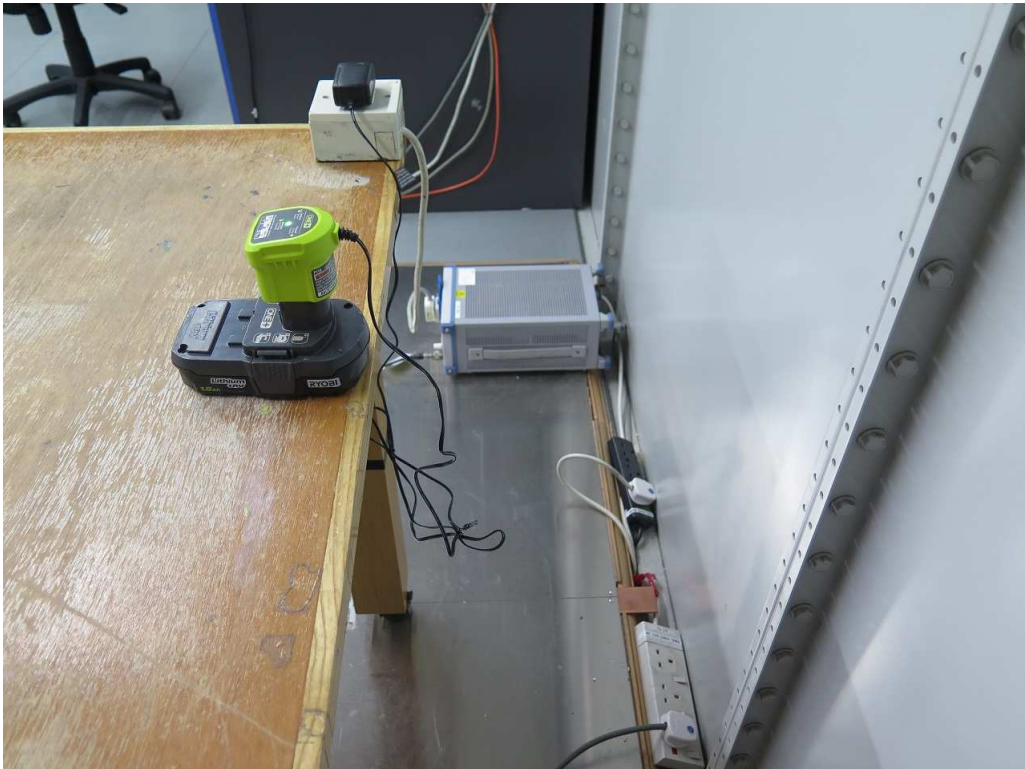
Line-conducted emission (rear view, charging)
