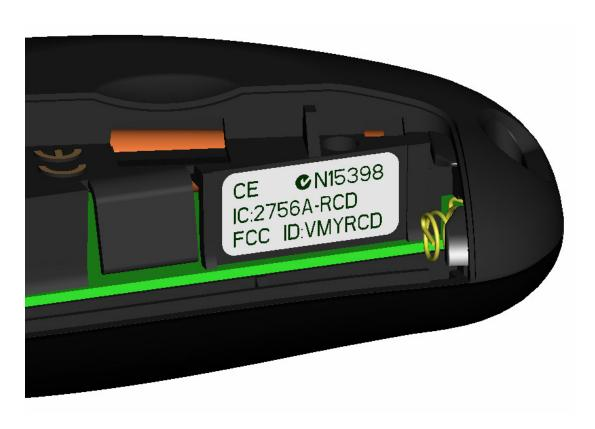
The label is placed within the battery compartment of the device
