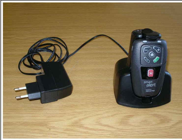
Smart Alert mounted on charging station with external power supply
