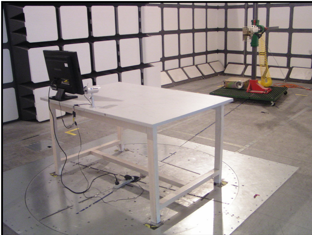
Radiated Emissions - Rear View (Above 1 GHz)
