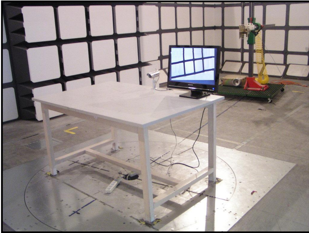
Radiated Emissions - Rear View (Above 1 GHz)
