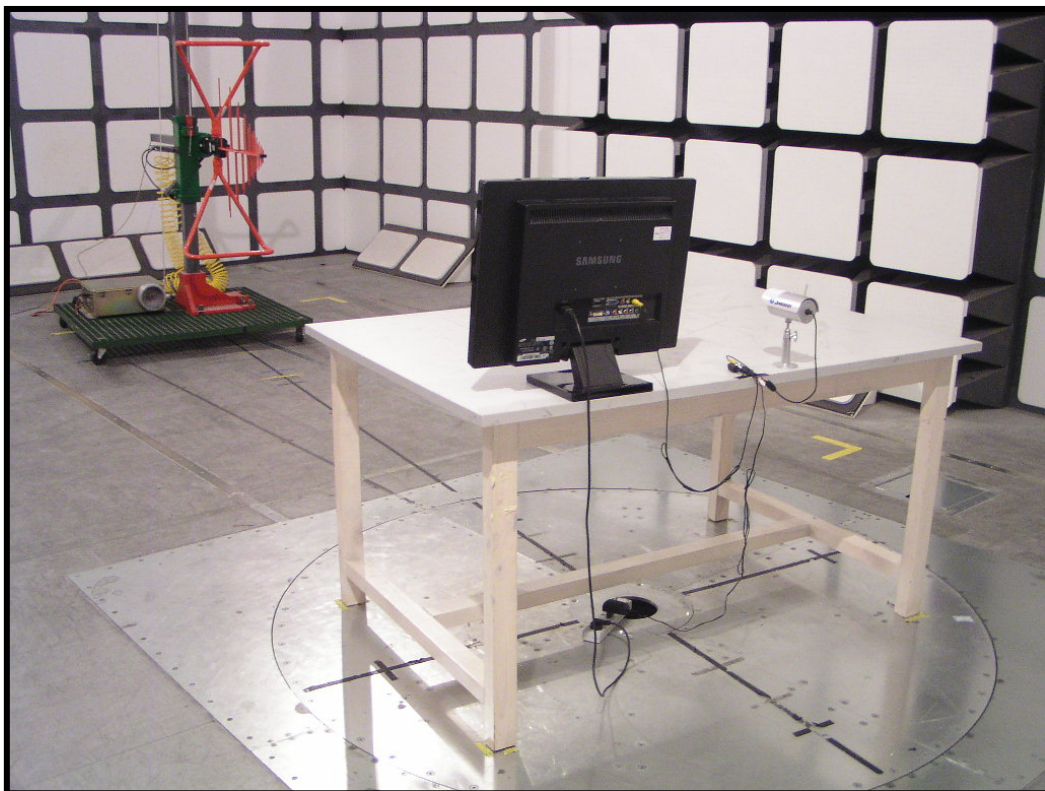
Radiated Emissions - Rear View (30 MHz-1 GHz)
