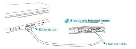
The Ethernet cable is only required for initial setup. Configure the Smart Hub to connect to your Wi-Fi network directly during registration then go wireless.
