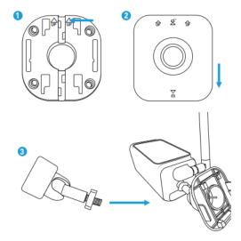
Securely attach the camera to a level surface using the included screws and wall plugs. Ensure that the surface is sturdy nough.
