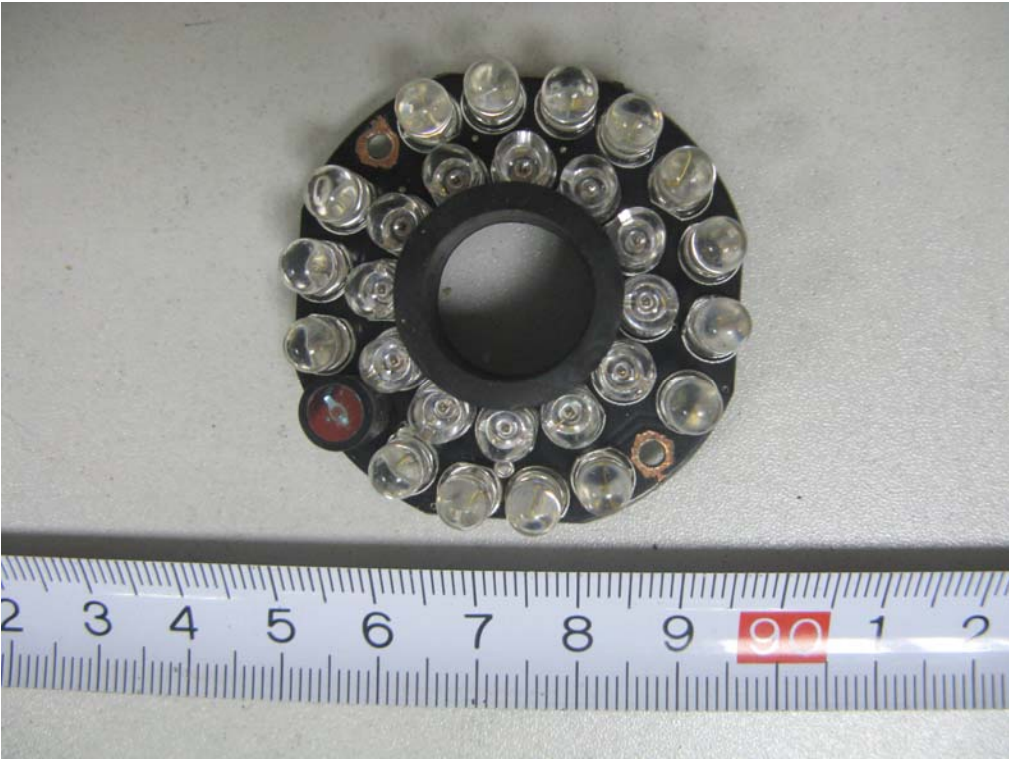
EUT – LED Board Top Components View
