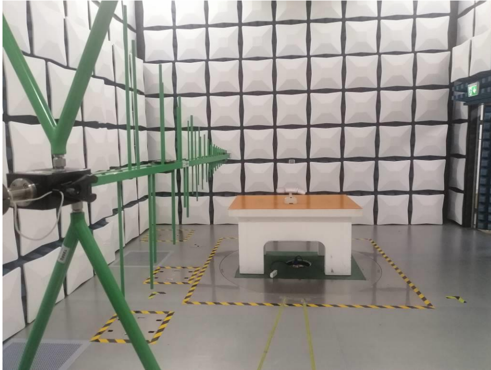
Photographs 1-2: Set-up for Field strength of fundamental and Unwanted Emissions in the Spurious Domain
