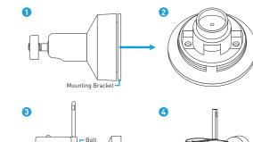
The camera can be mounted onto a flat surface using the screws and wall plugs provided. The surface must have sufficient strength to hold the camera.
