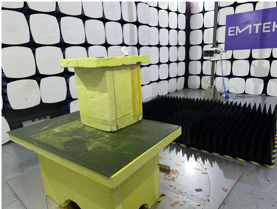
Spurious Emission Test Setup (Above 1GHz)
