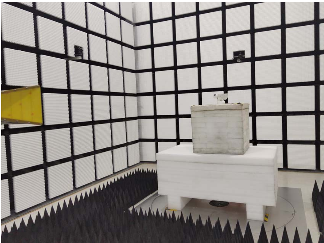
Radiated Emission Above 1GHz View
