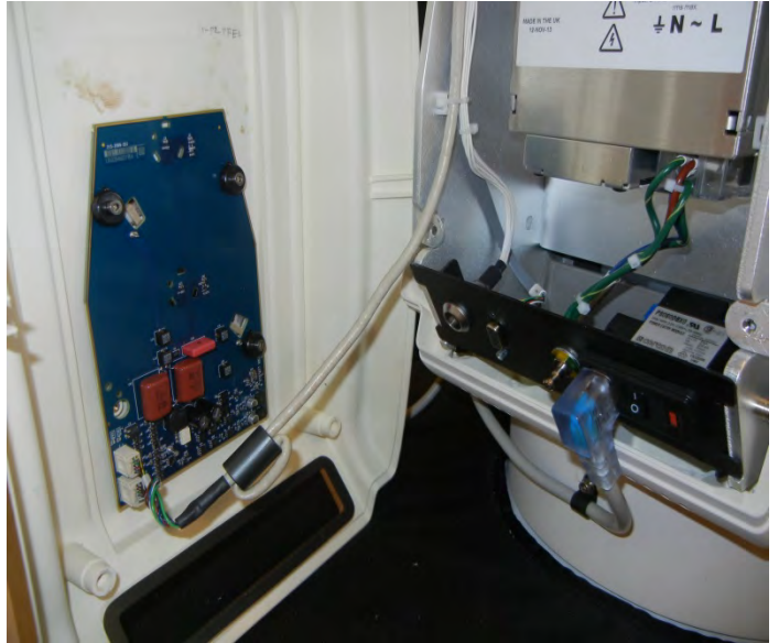
LuxOR Microscope Rear Panel Open, Charger PCB Mounting
