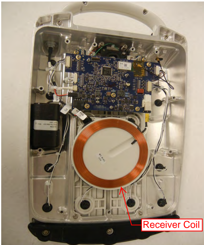
LuxOR Microscope Foot Controller Open - bottom view
