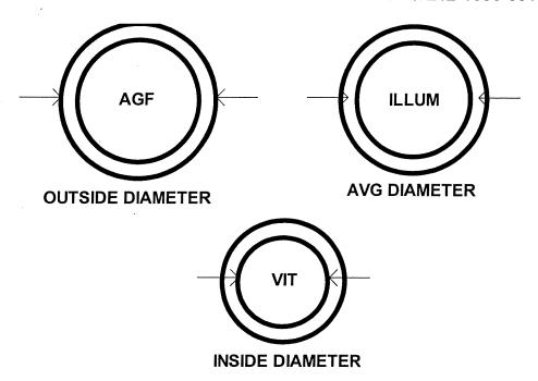
The Pneumatics RFID PCBA (212-1621-501) has 7 antennas, 6 of which are identical in size (marked VIT above). The 7th antenna is marked AGF above (largest of the 3). The Illuminator RFID PCBA (212-1630-501) has two antennas, identical in size (marked ILLUM above).
