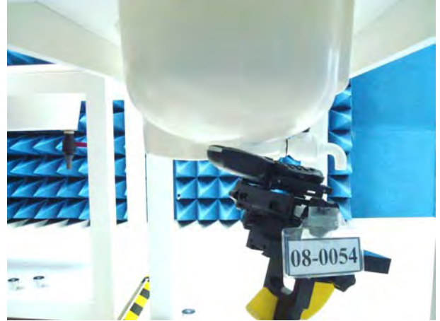
Figure 14.Right Head SAR Test Setup (Tilted)
