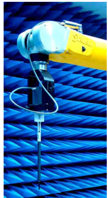
Figure 7. Probe setup on robot
