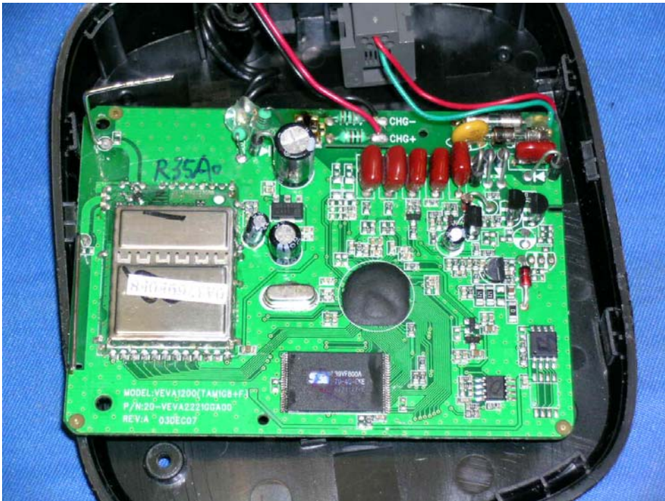
Base Unit Main PCB comp side
