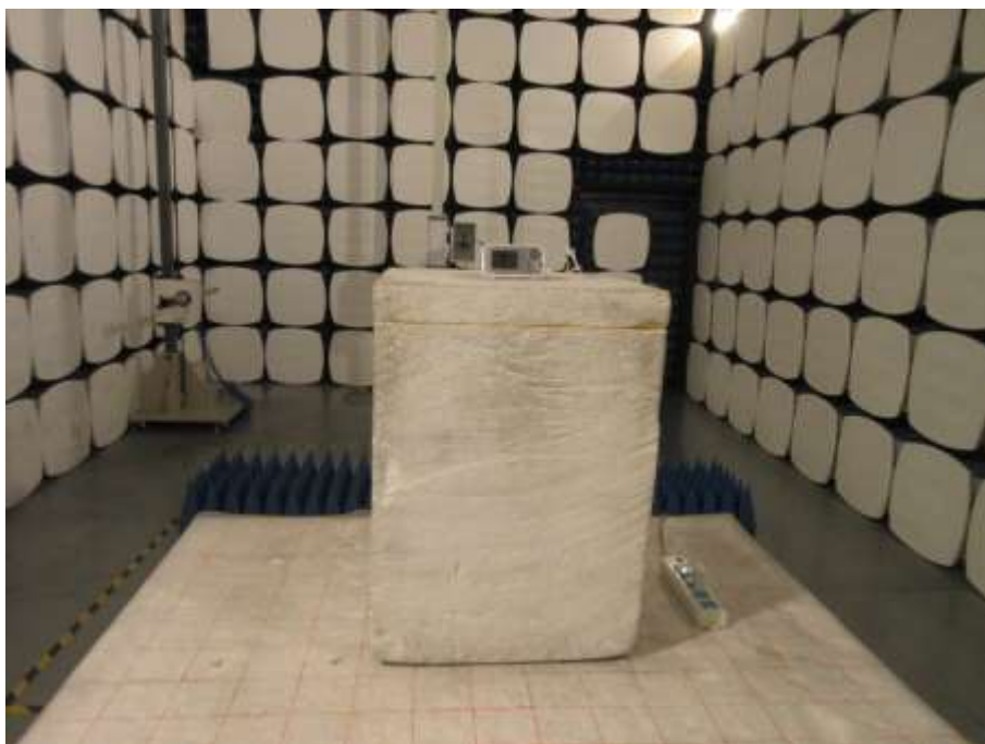
Radiated SPURIOUS EMISSION SET-UP PHOTOS, 1GHz ~ 25GHz
