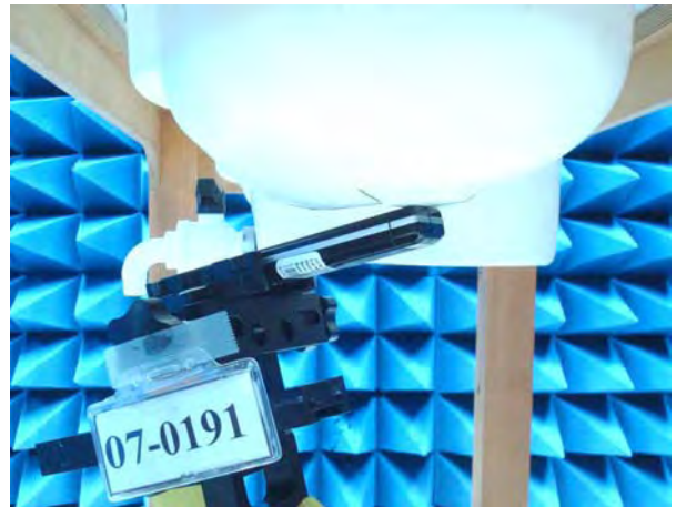
Figure 16. Left Head SAR Test Setup (Tilted)
