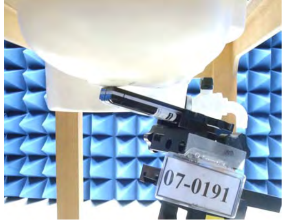
Figure 14. Right Head SAR Test Setup (Tilted)
