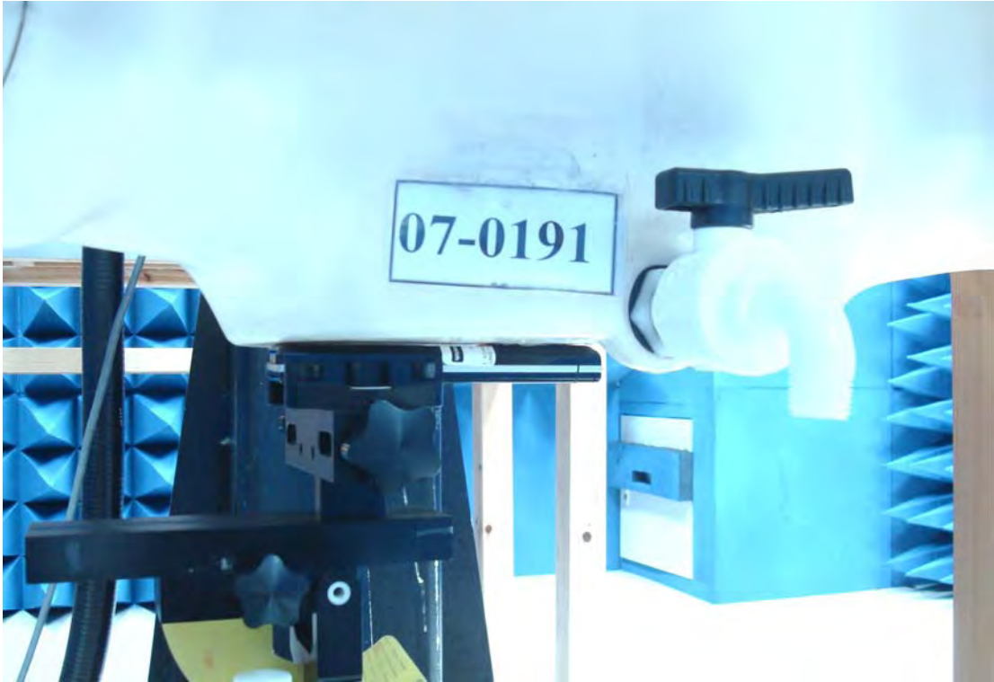
Figure 17. Body SAR Test Setup_ (Flat Section)
