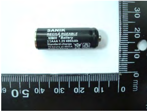
Figure 2. Battery (Ni-MH 1.2V , 400mAh)
