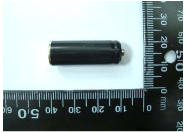
Figure 2. Battery (Ni-MH 1.2V , 400mAh)
