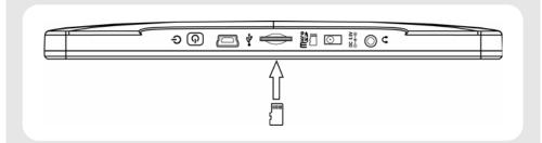
1. Insert the memory card into the card slot in the direction as indicated above until it clicks into place.
