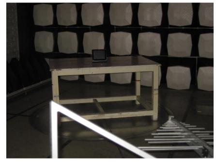
Radiated Spurious Emission Test Setup
