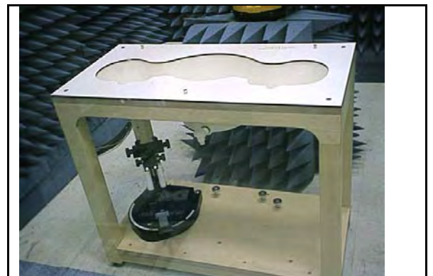
Figure 6. SAM Twin Phantom
