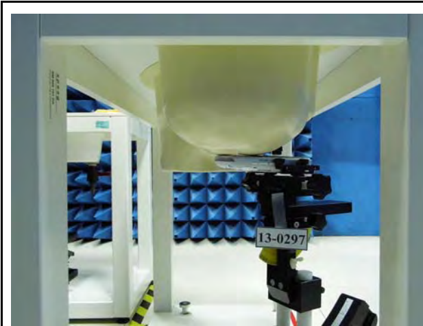
Figure 2. Right Head SAR Test Setup (Cheek)
