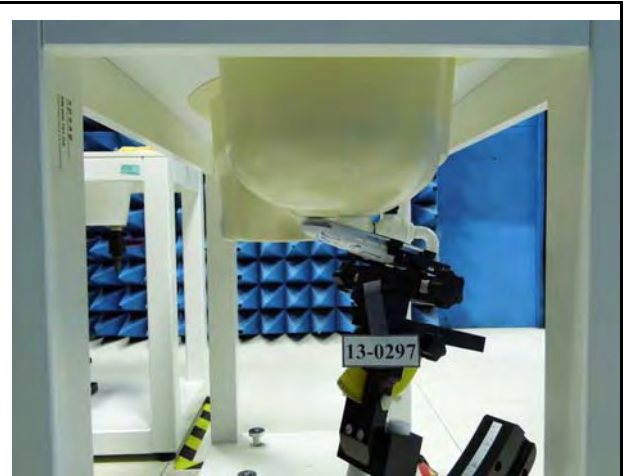
Figure 3. Right Head SAR Test Setup (Tilted)
