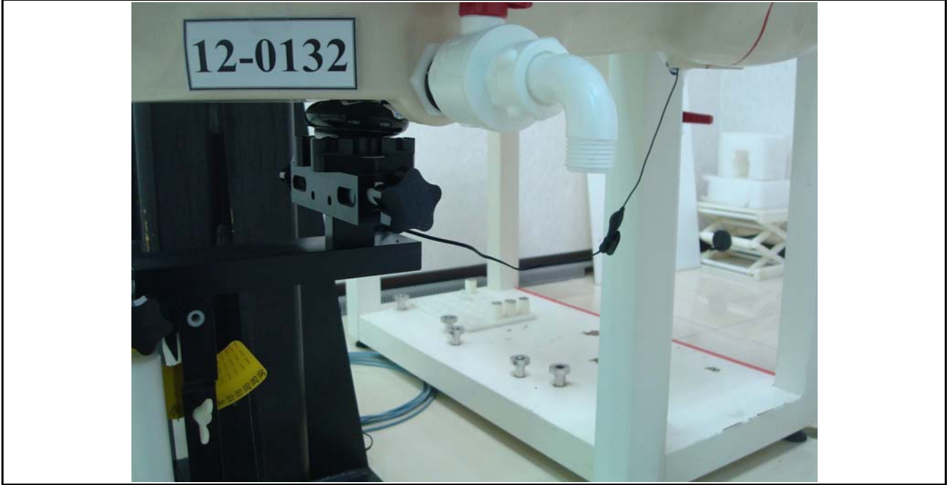
Figure 2. Body SAR Test Setup (Flat Section)
