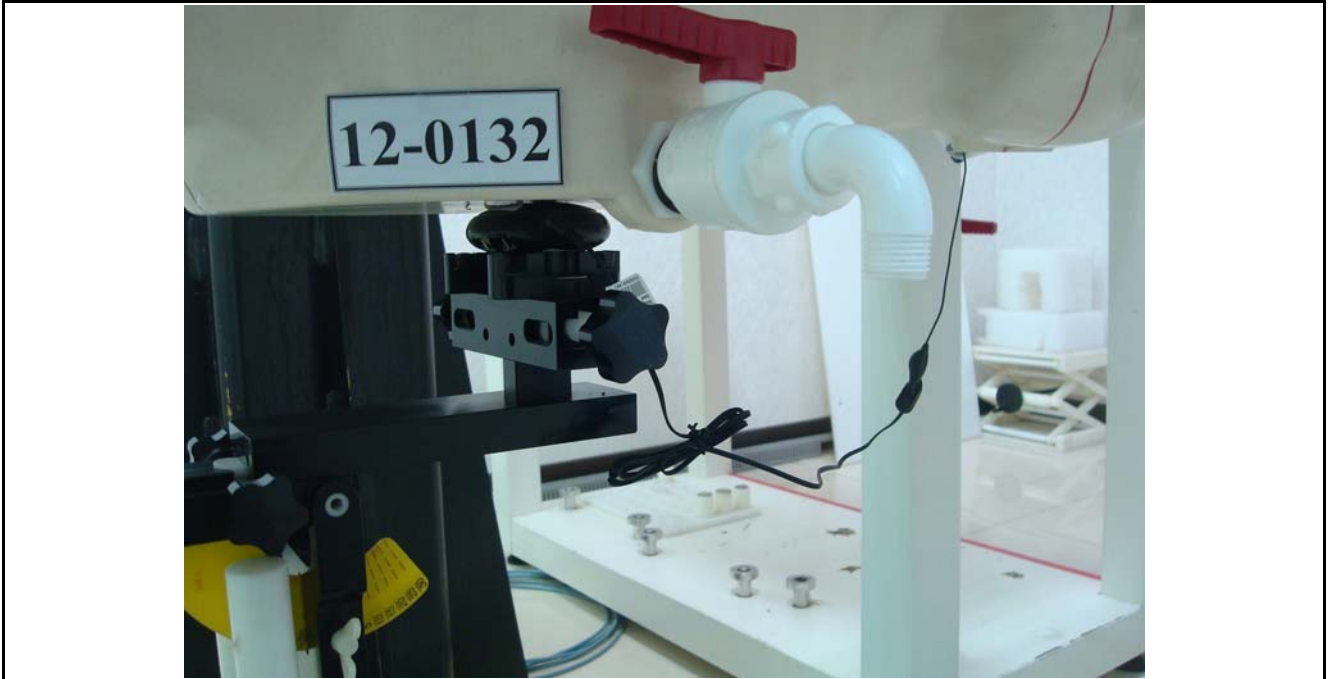
Figure 3. Body SAR Test Setup (Flat Section)
