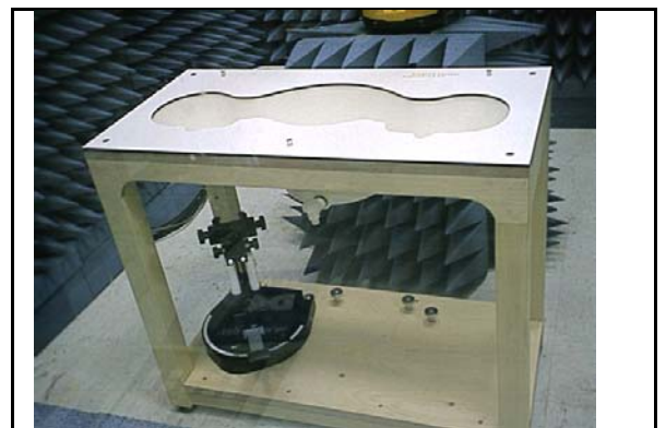
Figure 6. SAM Twin Phantom
