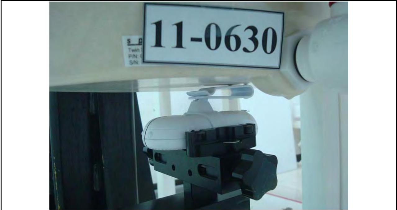
Figure 4. Body SAR Test Setup (Flat Section)
