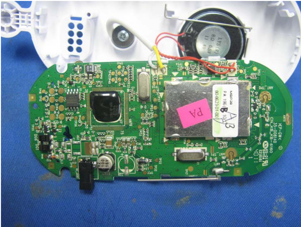
Baby Unit Main PCB comp side
