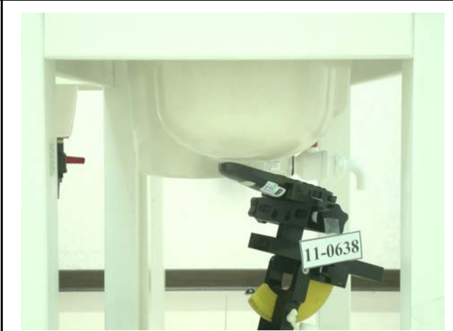
Figure 3. Right Head SAR Test Setup (Tilted)
