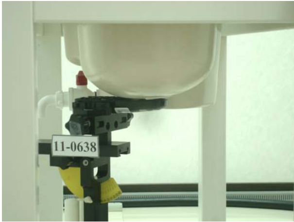
Figure 4. Left Head SAR Test Setup (Cheek)
