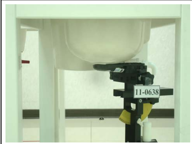
Figure 2. Right Head SAR Test Setup (Cheek)
