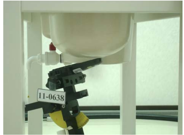
Figure 5. Left Head SAR Test Setup (Tilted)
