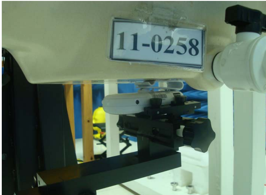
Figure 2. Muscle SAR Test Setup (Flat Section) _ Surface Back to phantom
