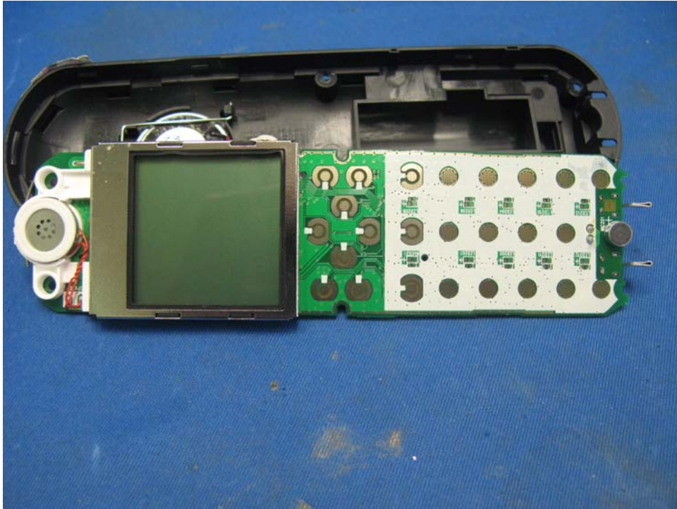
Handset Main PCB display side (View 1)
