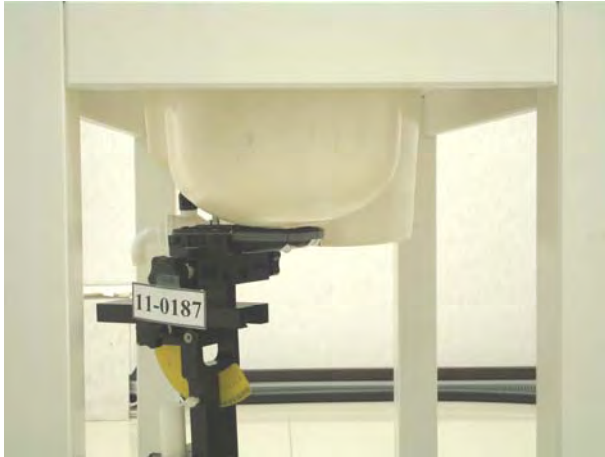
Figure 4. Left Head SAR Test Setup (Cheek)
