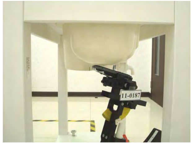
Figure 3. Right Head SAR Test Setup (Tilted)
