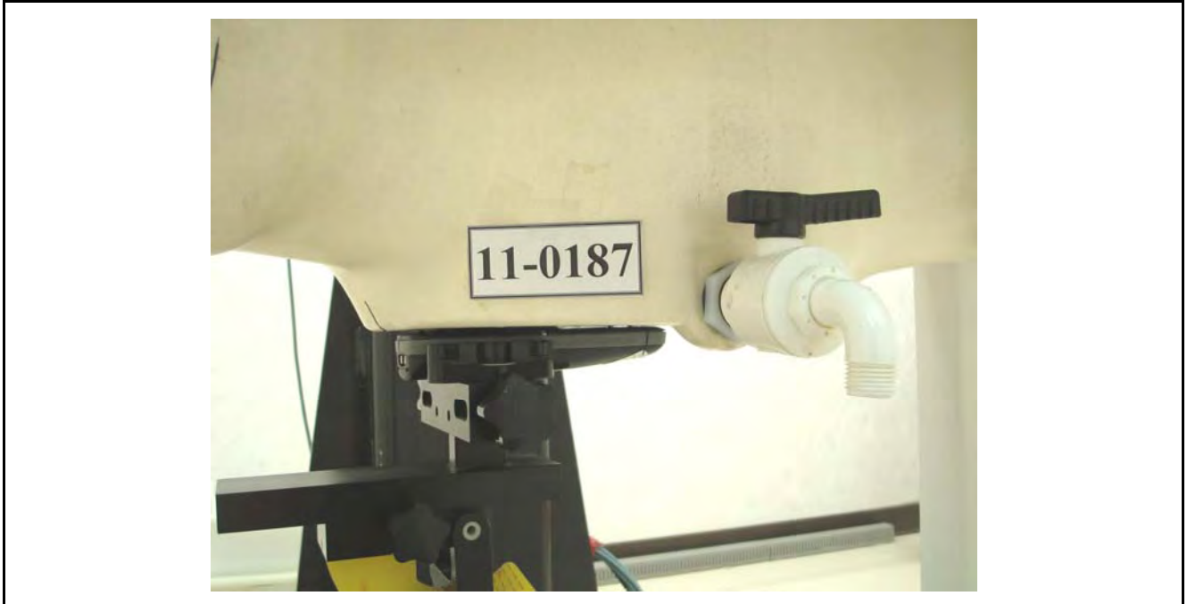
Figure 6. Body SAR Test Setup (Flat Section)
