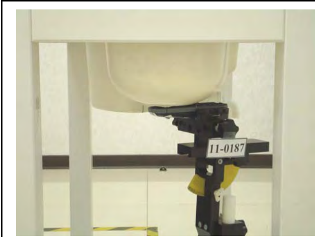
Figure 2. Right Head SAR Test Setup (Cheek)
