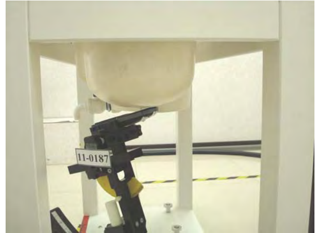
Figure 5. Left Head SAR Test Setup (Tilted)
