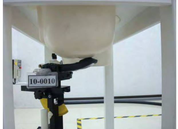
Figure 5. Left Head SAR Test Setup (Tilted)
