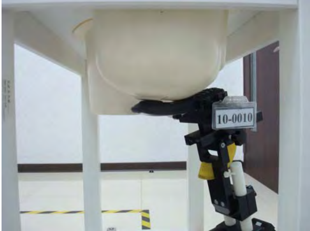
Figure 2. Right Head SAR Test Setup (Cheek)
