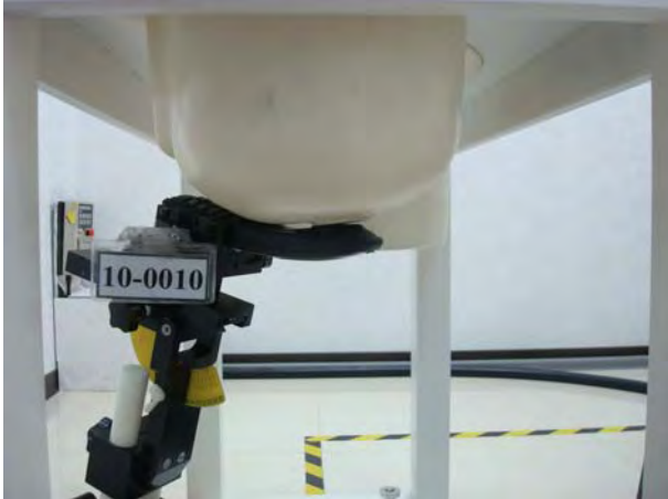
Figure 4. Left Head SAR Test Setup (Cheek)
