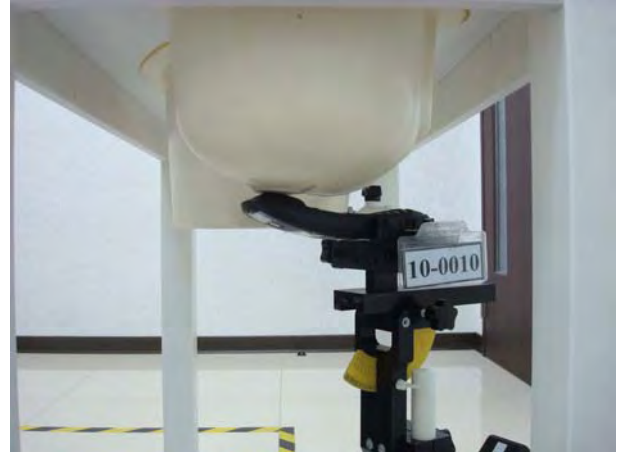
Figure 3. Right Head SAR Test Setup (Tilted)
