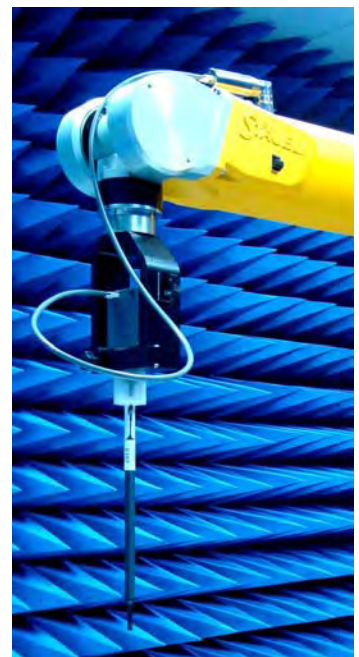
Figure 5. Probe setup on robot
