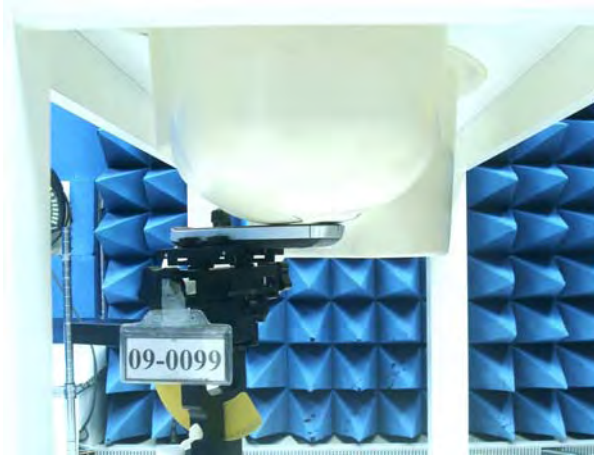
Figure 16. Left Head SAR Test Setup (Cheek)
