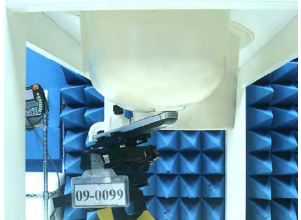
Figure 17. Left Head SAR Test Setup (Tilted)
